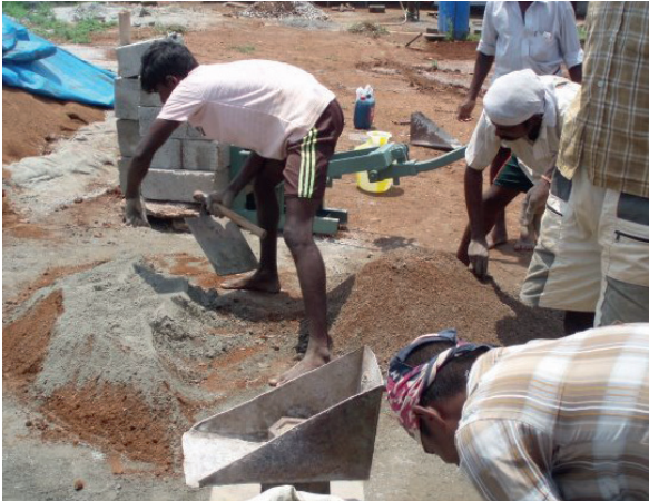
Fig. 5 Typical CSSB block production unit
