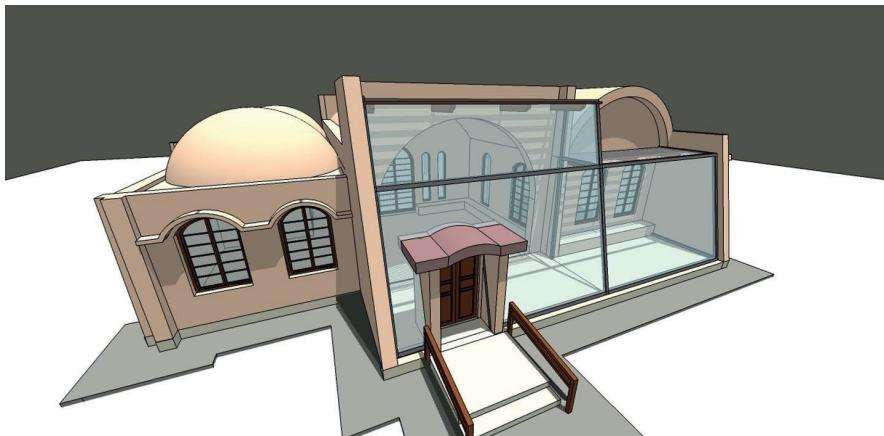
This design is based on the NM earth construction code; wall construction using natural, non-stabilized 14-inch adobe walls on gravel trench ground-beam foundations. The roofing system uses domes and vaults, based on what is generally called the Nubian vault style. It is highly seismic resistant, which is more easily adaptable to the site and is a very appropriate architectural style for the Syrian Central Plateau.
