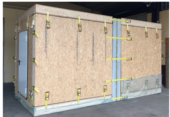
Fig. 9 Mobile sound test facility
