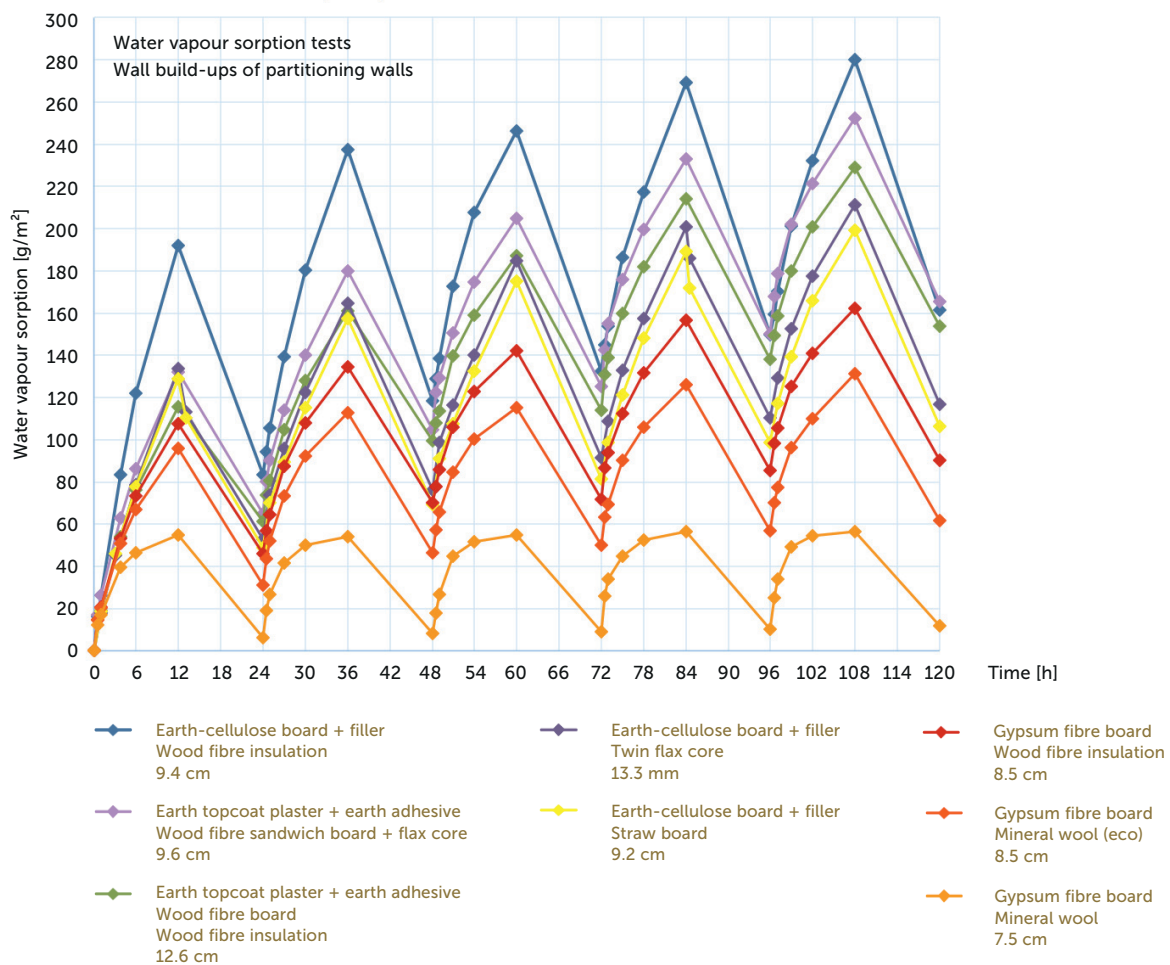
Fig. 6 Results of the water vapour sorption tests (five cycles ad- and desorption) of wall build-ups
