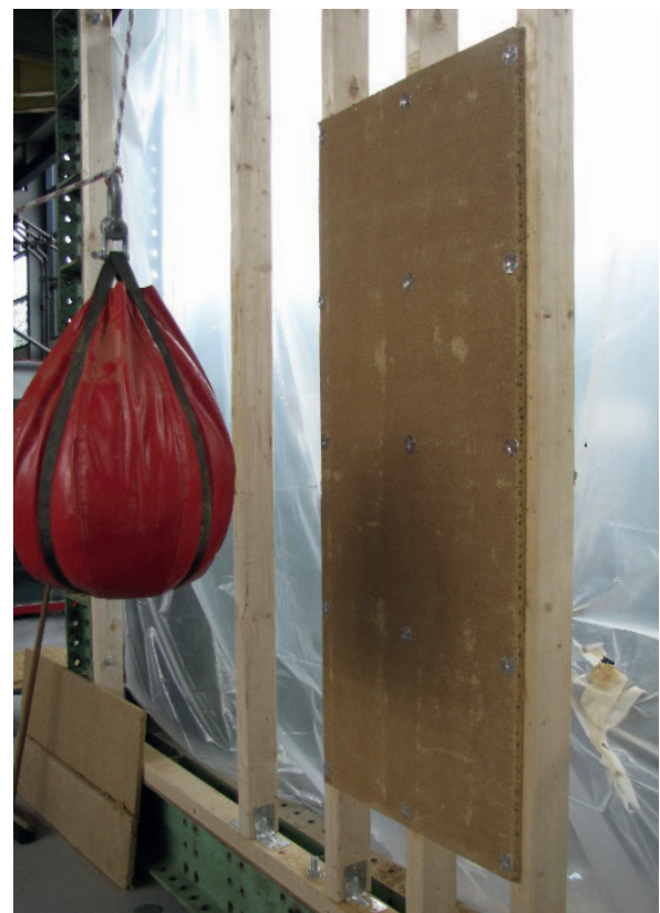
Fig. 2 Test stand for the conduct of the soft impact according to DIN 4103-1 [9].
