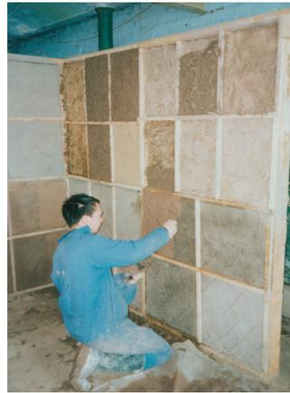
finishes. The programme produced unexpectedly good and bad results in a number of tests and these indicated that some of the interactions between materials are complex and not fully understood.
